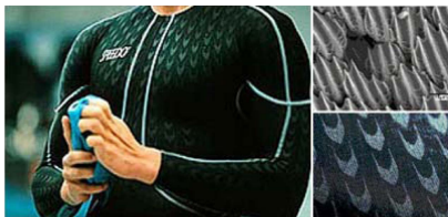
Fig. 13. Fast skin suit of Speedo. up: protuberance of shark, down: surface of fast skin http://web.mit.edu .
