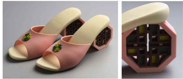
Fig. 14. 3D printed shoes made utilizing traditional muntin patterns.
