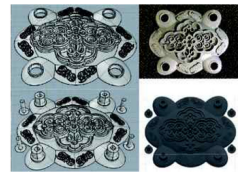
Fig. 11. The images of 3D models and printed objects by SLA based on 'Taepyongwha' pattern (August 14, 2018).
