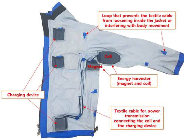
Fig. 8. Inner appearance of a jacket with pockets for energy generation, storage and charging devices.
