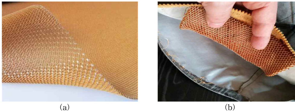
Fig. 1. Honeycomb structured aramid (a) and honeycomb structured aramid layered in firefighters' protective clothing in the present study (b).
