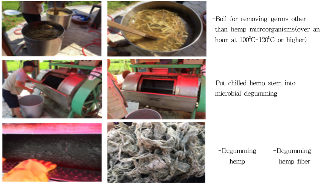
Fig. 6. Microbial degumming process of hemp.
