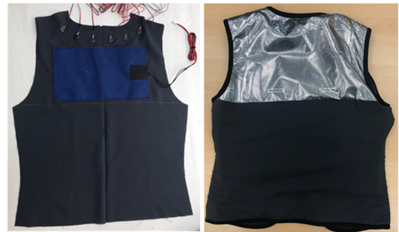
Fig. 9. Device location and lining of vest.
